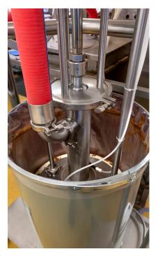
months of operation, this system is proving to be reliable and simple to operate. It presents the advantage of being air-operated, which avoids many washing restrictions due to the absence of electricity," observes Eric Bruncher.
